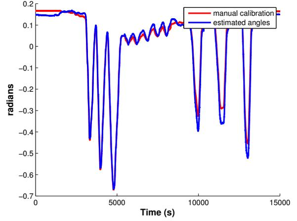
Fig. 4: Estimated joint angle by optimization
