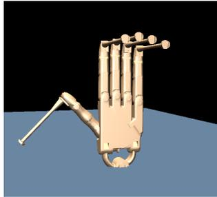
(a) MuJoCo Hand Model with Kinematic Extensions
