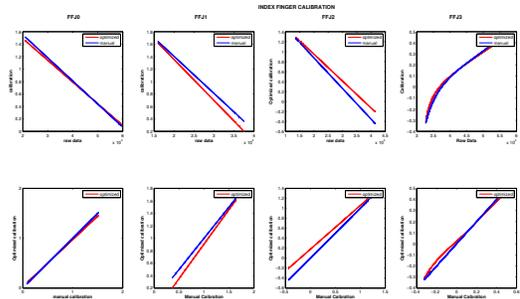
Fig. 6: Index finger, manual and optimized calibration
