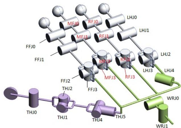
Fig. 1: Kinematic Structure of Shadow hand
