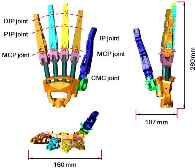
Fig. 2: 3D model of the anthropomorphic robotic hand.
