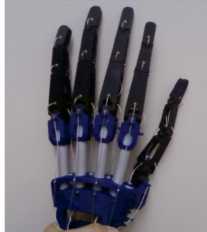
Fig. 1: The 3D-printed 20-DOF anthropomorphic robotic hand.
