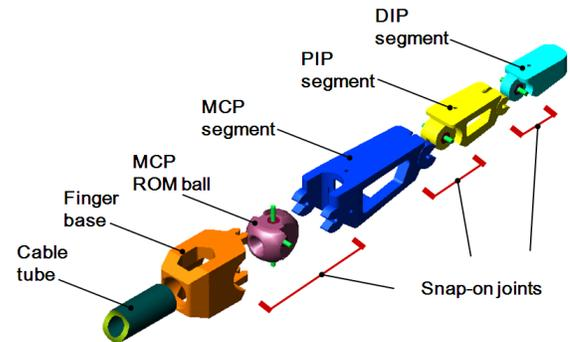
Fig. 3: Components of each finger unit.
