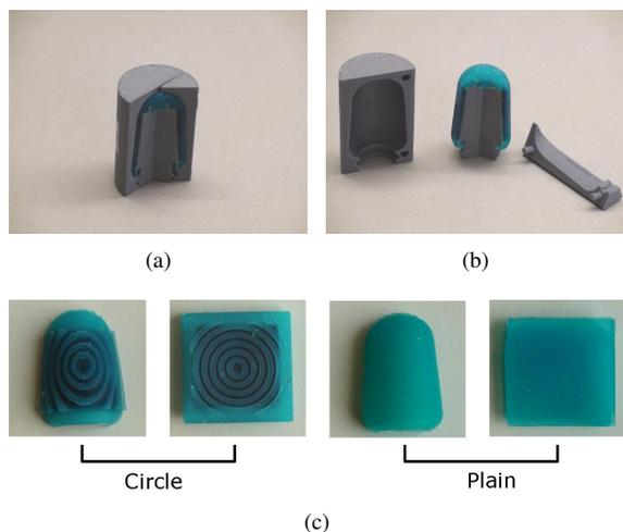
Fig. 7: The prototyping process of the artificial skin. *Top row:* Components of the molds used for prototyping the fingertip's skin. *Bottom row:* Skin pads with different textures on two types of skin shapes.
