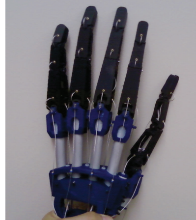
Fig. 1. The 3D-printed 20-DOF anthropomorphic robotic hand.
