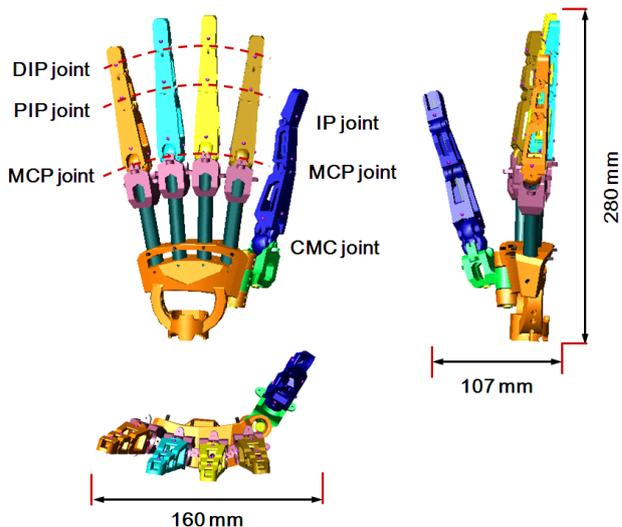
Fig. 2: 3D model of the UW hand.
