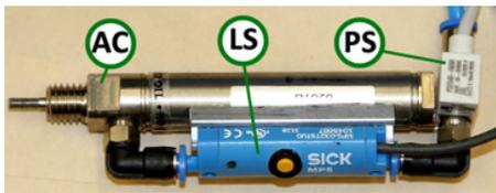
Fig. 7: Cylinder unit (AC: Actuator, LS: Length Sensor, PS: Pressure Sensor)
