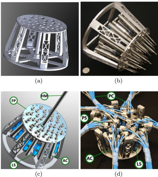
Fig. 8: Housing assembly (a) CAD model of the bracket; (b) Cylinders pointing to the wrist opening; (c) Housing assembly in CAD model; (d) Final assembly (without back plate). (FP: Front Plate, HM: Hand Mount, LS: Length Sensor, AC: Actuator, PS: Pressure Sensor)
