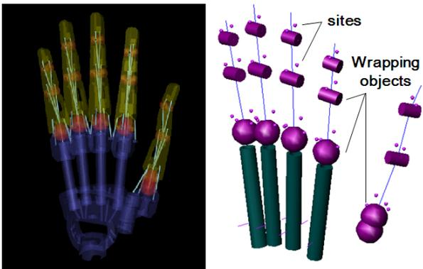
Fig. 10: MuJoCo model of the UW hand. *Left:* kinematic model of the robotic hand visualized in OpenGL. *Right:* The model of the cable paths.
