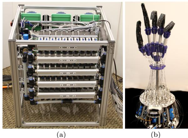
Fig. 9: The actuation system of the UW Hand. *Left*: the pneumatic control unit. *Right*: Fully assembled UW Hand.
