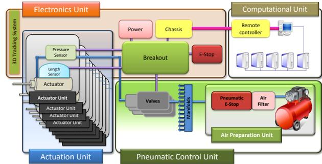
Fig. 6: Schematic drawing of the actuation system.
