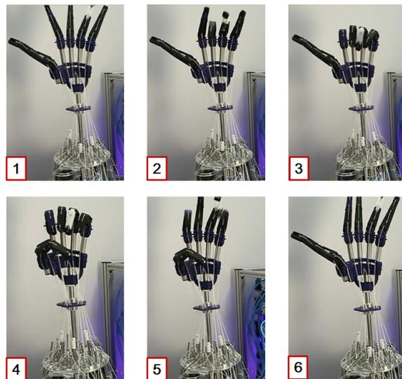
Fig. 13: The sequence of images of the UW hand performing envelop grasp.
