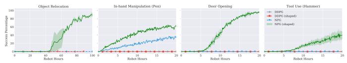
Figure 7: Performance of pure RL methods – NPG and DDPG, with sparse task completion reward and shaped reward. Sparse reward setting is primarily ineffective in solving our task set (expect in-hand manipulation). In corporation of human priors in-terms of reward shaping helps NPG get off the ground, but DDPG sill struggles to find success.
