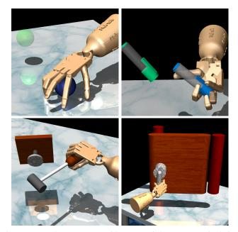
Figure 1: We demonstrate a wide range of dexterous manipulation skills such as object relocation, in-hand manipulation (pen repositioning), tool use (hammering a nail), and interacting with human centric environments (opening a door) using DRL methods. By augmenting with human demonstrations, policies can be trained in the equivalent of a few real-world robot hours.
